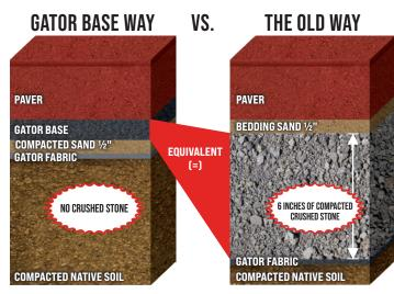
GATOR BASE REPLACES 6" OF COMPACTED CRUSHED STONE!
