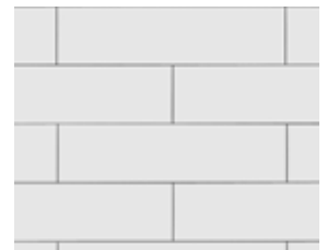
BROKEN BOND INSTALLATION
